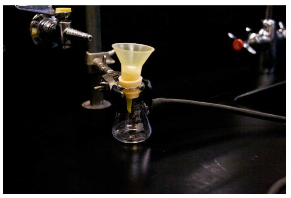
Note that the thin hose is connected to the vacuum hose on the faucet – the vacuum hose is always the "arm" hose of the faucet; DO NOT connect to the vertical water hose or you will fill your filtering flask up with water!
